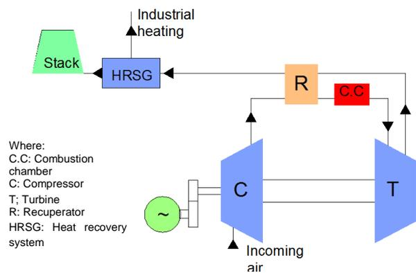
Figure 1.Schematic view of amicroturbine system
