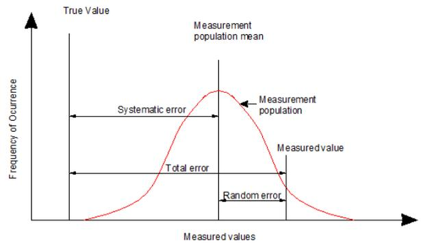
Figure 5. Components of total error [7]
