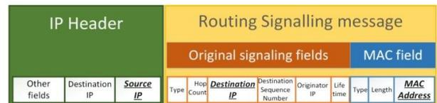
Figure 1. An IP Packet carrying a VANET Routing signaling message
