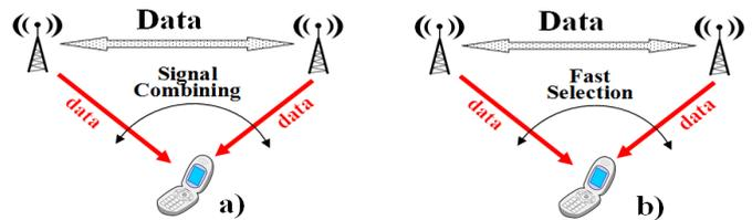
Figure 6. Joint processing techniques: a) joint transmission b) dynamic cell selection (Akyildiz et al., 2010).
