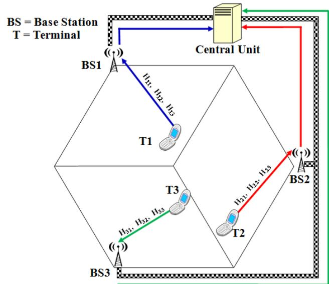
Figure 3. CoMP centralized architecture (Akyildiz et al., 2010).
