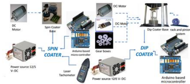
Figure 7. An overview of the mechanical and electronic components used.
