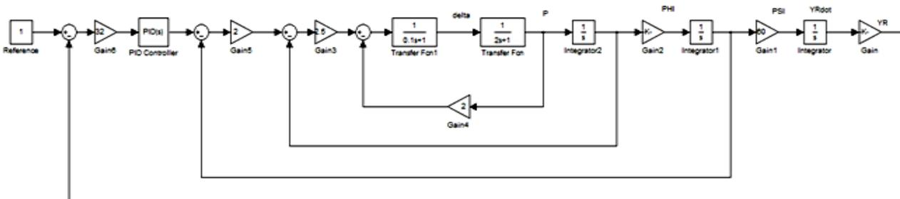
Figure 5.Block diagram of an aircraft directional-control system
