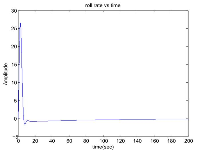
Figure10. Roll rate  $p$  when the reference is 15 degrees without controller
