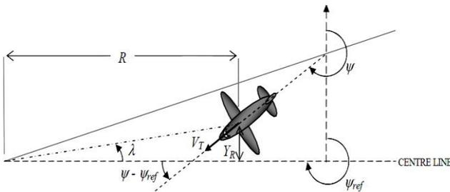
Figure4.System of Lateral Beam Guidance
