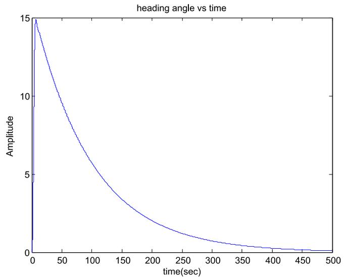
Figure8. The heading angle  $\psi$  when the reference is 15 degrees without controller
