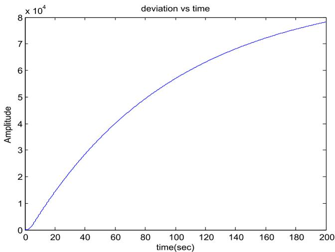
Figure7. The deviation YR when the reference is 15 degrees without controller
