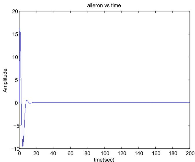
Figure 11. aileron deflection  $\delta$  when the reference is 15 degrees without controller
