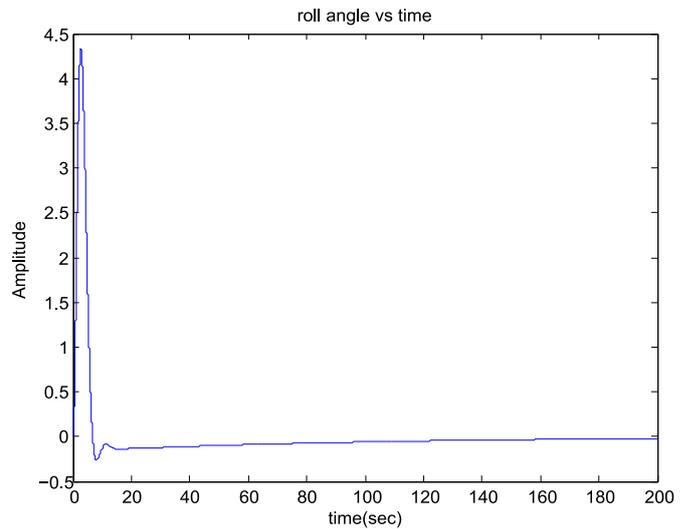
Figure 9. Roll angle  $\psi$  when the reference is 15 degrees without controller
