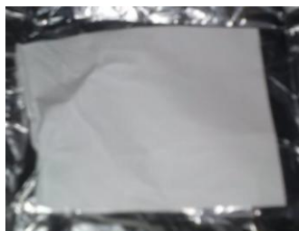
Figure 2. Mat formed through electrospinning test.
