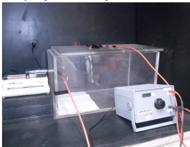
Figure 3. Scheme of electrospinning test.
