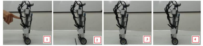
Figure 11. Dynamic behavior of the robot with an external back force.
