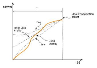
Figure 4. Energy consumption curve and its maximum and minimum limits. (Load management with Ekip power controller for SACE Emax 2, 2012).
