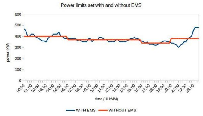
Figure 9. Configuration profile of the power limits in the EMS controller with and without using the EMS tool.
