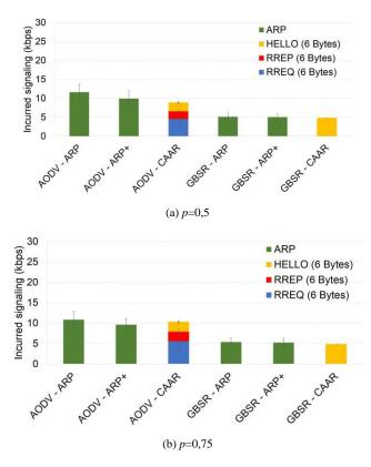
Figure 5. Signaling traffic incurred only by the AR process in our Crowdslike anonymity service scenario using the three Address Resolution schemes (CI 95 %). AR signaling in ARP and ARP+ involves all ARP REQ/REP messages. AR signaling in CAAR only consists of 6 bytes added to each routing message (RREQ, RREP and HELLO in AODV and HELLO in GBSR) to carry the MAC address.
