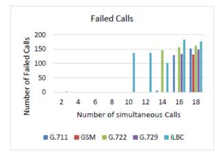
Figure 6. Failed calls per codec and number of simultaneous calls
