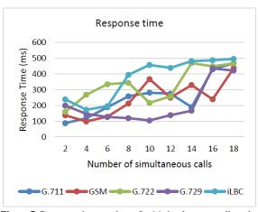
Figure 7. Response time varying – for 14 simultaneous calls and using G.729
