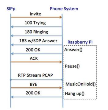
Figure 2. Call flow used to evaluate the performance of the IP telephony
