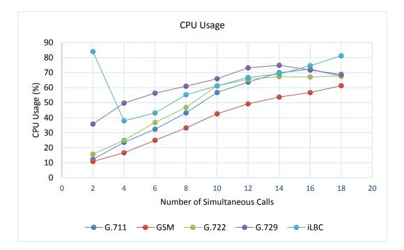
Figure 1. Percentage of CPU usage according to the codec used and the load of the system in terms of the number of simultaneous calls
