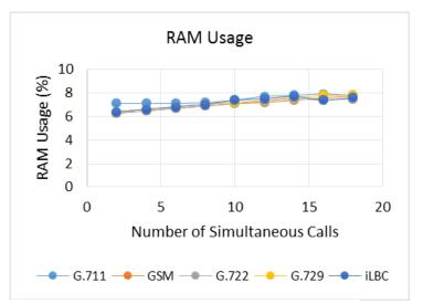
Figure 3. Percentage of RAM used during the test of the system, for different codecs and number of simultaneous callssystem based on the Raspberry Pi platform
