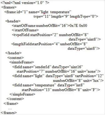
Figure 6. The frame description for the raw frame in Figure 5
