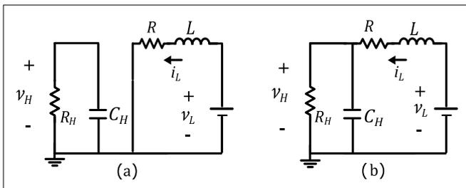
Figure 3. Boost operation: (a) ON state: Q<sub>2</sub> ON – Q<sub>1</sub> OFF, (b) OFF state: Q<sub>2</sub> OFF – Q<sub>1</sub> ON
