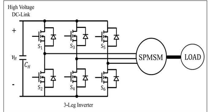
Figure 5. Inverter and electric machine configuration
