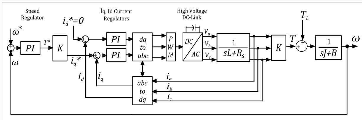
Figure 6. Cascade control scheme for the SPMSM
