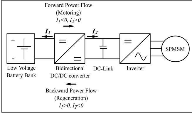
Figure 1. General scheme for electric vehicle applications
