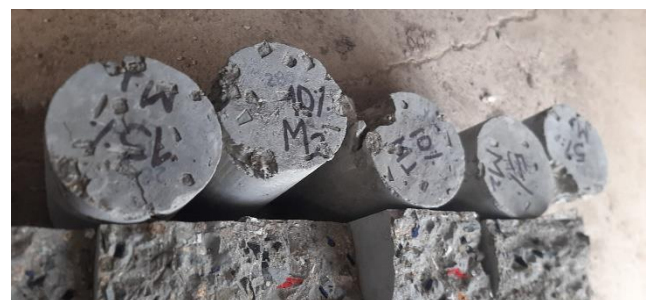
Figure 2. Mode of failure of cylinders and beams after breakage
